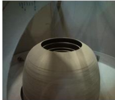
Şekil 4. 1200 kV Exit Insulation System located in Power Transformer Turret.
