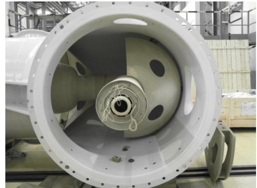
Şekil 7. 765 kV Exit Insulation System located in Power Transformer Turret
